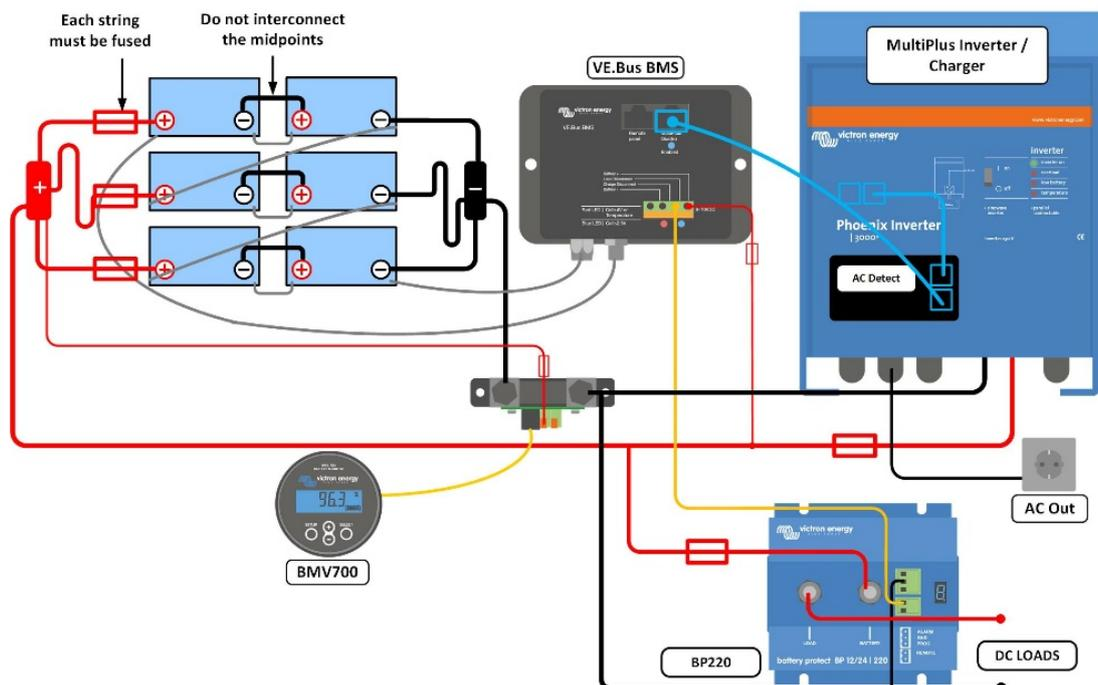
Our LFP batteries have integrated cell balancing and cell monitoring. Up to 5 batteries can be paralleled and up to four batteries can be series connected, so that a 48V battery bank of up to 1500Ah can be assembled. The cell balancing/monitoring cables can be daisy-chained and must be connected to a Battery Management System (BMS).
