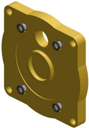
Figure 8: 7170 Maintenance Small Housing O-Rings Close-up
