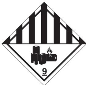
Use Class 9 Miscellaneous Dangerous Goods and UN Identification labels for transportation of Lithium-ion batteries which are assigned Class 9. Refer to relevant transportation documents. Lithium and Lithium-ion cells and batteries are regulated in the U.S. in accordance with Part 49 of the Code of Federal Regulations, (49 CFR Sections 105-180) of the U.S. Hazardous Materials Regulations.
